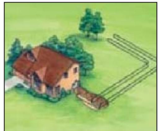
and carries the heat to the geothermal unit. The system amplifies the heat and delivers it indoors. The process is reversed in warm weather, with excess heat carried from indoors and delivered into the earth.
